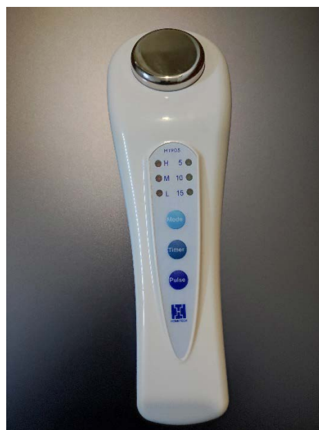
Figure 2: Portable therapeutic ultrasound machine (Home Care Technology Co, Ltd, Taiwan)
